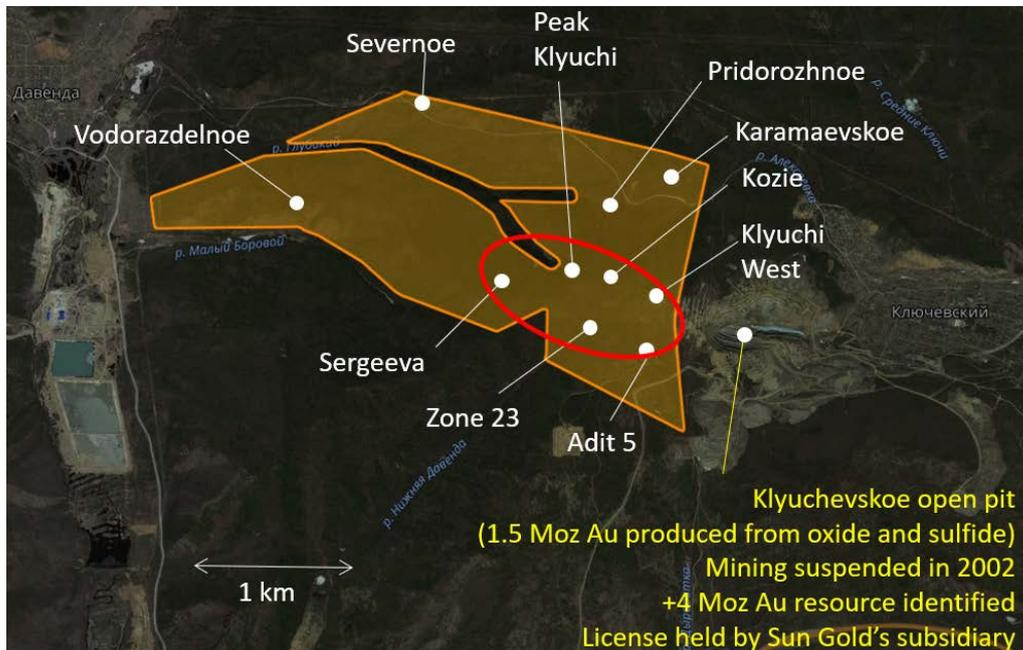
Figure 1. An outline of the 7.6 sq km Sergeevskoe license area with location of principal gold prospects and adjacent Klyuchevskoe open pit. The area of 2017-18 exploration works is shown in red.
