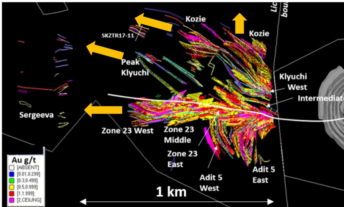
Figure 2. Plan view of the maiden Mineral Resource block model at Sergeevskoe and exploration targets at its western and northwestern extension. Grey-blue colours depict mineralized intercepts in the historical holes.
